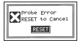
The probe is not connected or it is broken, check it then press ENTER to reset.
